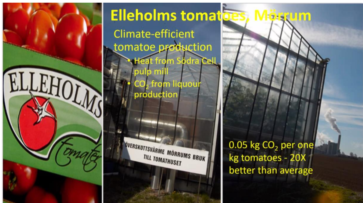
Figure 5 – Example of reconnection of industries – heat from a pulp mill and CO 2 from liquor production used at a greenhouse for the cultivation of tomatoes, which have a 20 times better CO 2 footprint than their common counterparts (Eklund).
