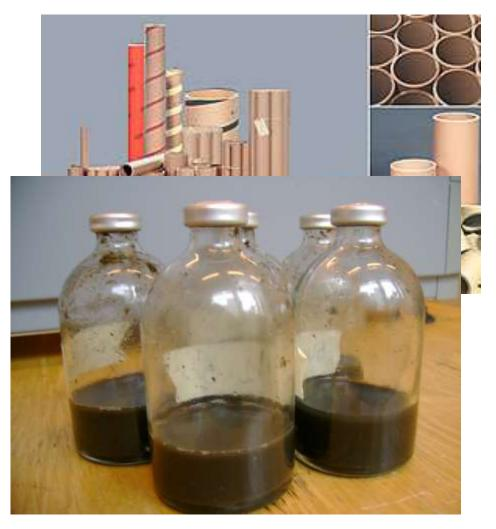
Methane production from untreated paper: 0.23 Nm<sup>3</sup> CH<sub>4</sub> /kg VS (≈ 200 Nm<sup>3</sup> CH<sub>4</sub> /ton dry paper)
